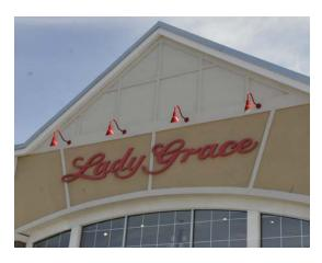
Small spotlights directed downward are easily aimed to prevent glare. The simple design of the fixture complements the line and colors of the sign.
